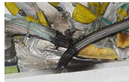
Damaged loom and hose 4
