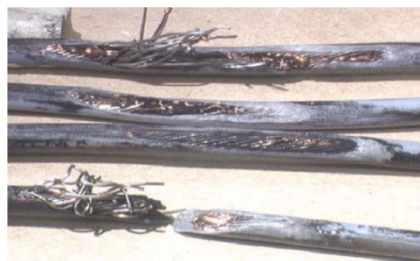
Damage to galley feeder cables 3
